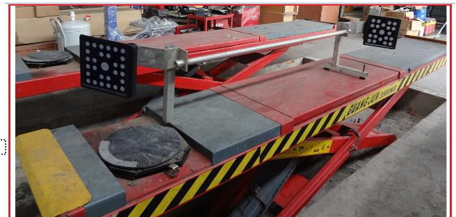
Step 1: put the calibration device on the left side of scissor lift
