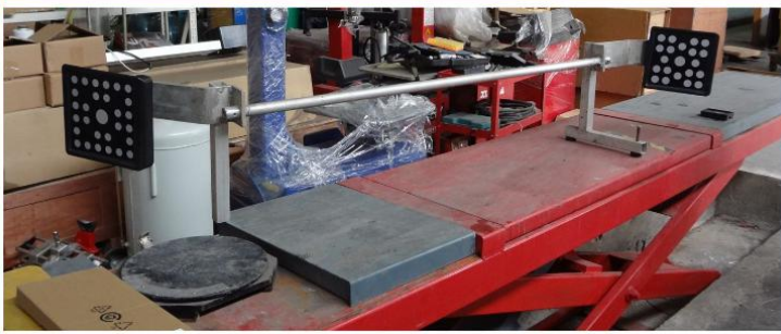
Step 4: put the calibration device on the right side of scissor lift
