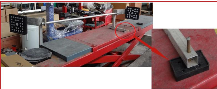
Step 5: put the small thing under the calibration device
